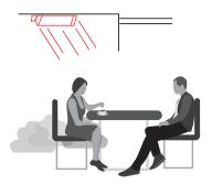
When outdoors, hang heater under protective roof or weather cover whenever possible. Even though heater is all-weather construction, it will last longer and look better if it is protected from rain and snow.
