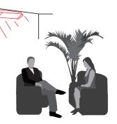
Install fixture to heat the area from the "cold side" if possible. This helps compensate for increased body heat losses due to exposure. Warm floors reradiate heat. Warmer air rises from floor. Some heat reflects from floor. Mounting a heater directly over a table or other obstruction will block the energy, primarily heating the object. It is best to move heater to the side, allowing complete body and floor coverage.
