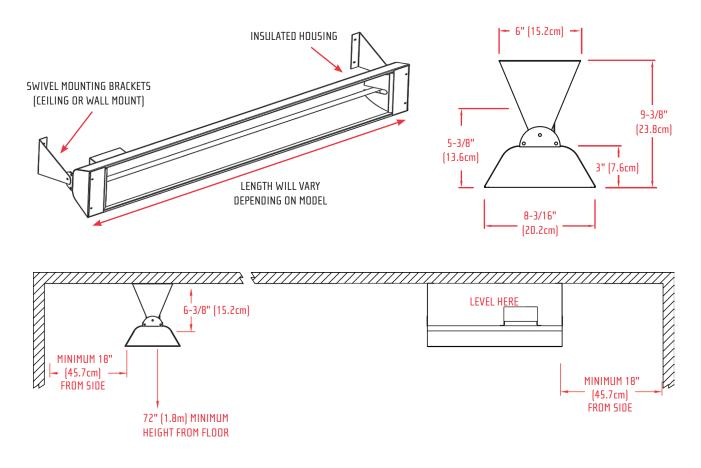
Heater must be installed with the quartz tube horizontally level. For maximum tube life, use a carpenter's level tool to find the optimum level position for the heater's body. Always maintain the minimum clearances from the heater body to any combustible materials.
